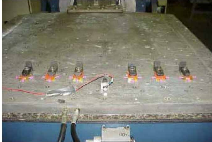
Figure 2-3. Test setup for longitudinal-axis Willoughby random vibration.
