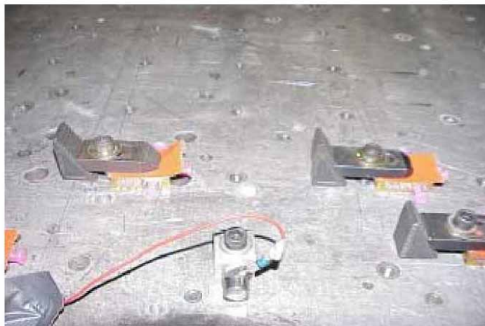
Figure 2-4. Test setup for lateral-axis Willoughby random vibration.
