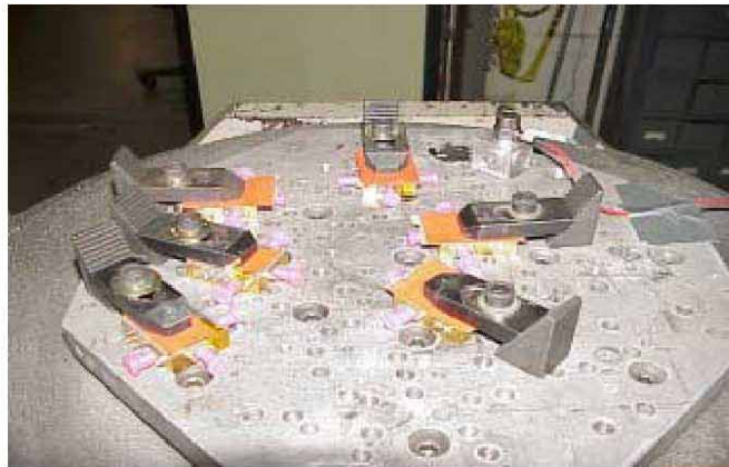
Figure 2-1. Test setup for vertical-axis bulkhead mounted level MPE random vibration.
