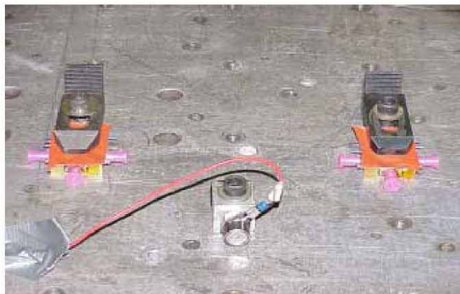
Figure 2-2. Test setup for longitudinal-axis bulkhead mounted level MPE random vibration.
