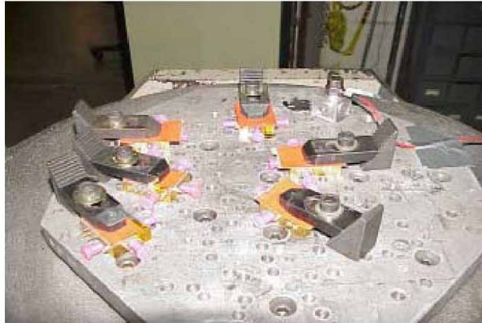
Figure 2-1. Test setup for vertical-axis Willoughby random vibration.
